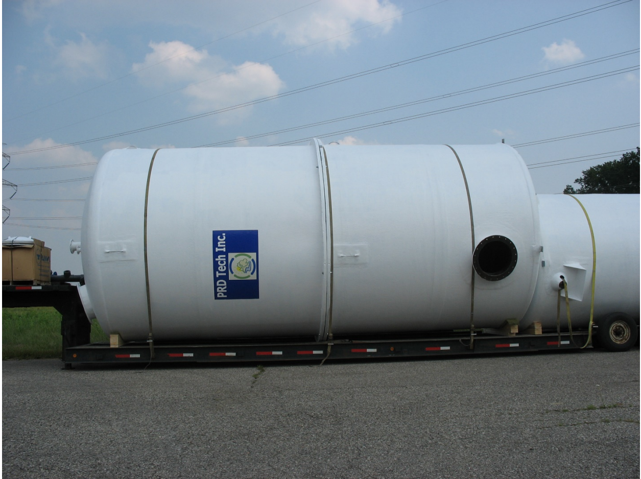
Magnesium Hydroxide tank to supply alkalinity for nitrification in bioreactor.
